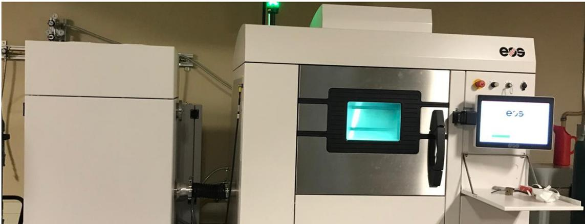
Figure 4-1: EOS M290 Direct Metal Laser Sintering Machine
