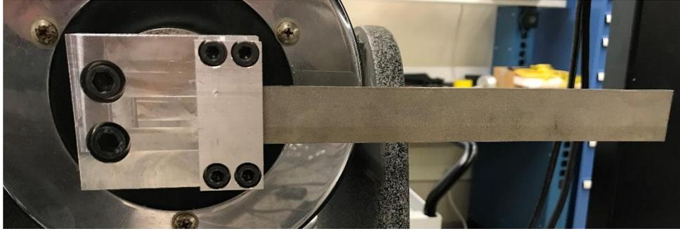
Figure 4-4: Beam Fixture
