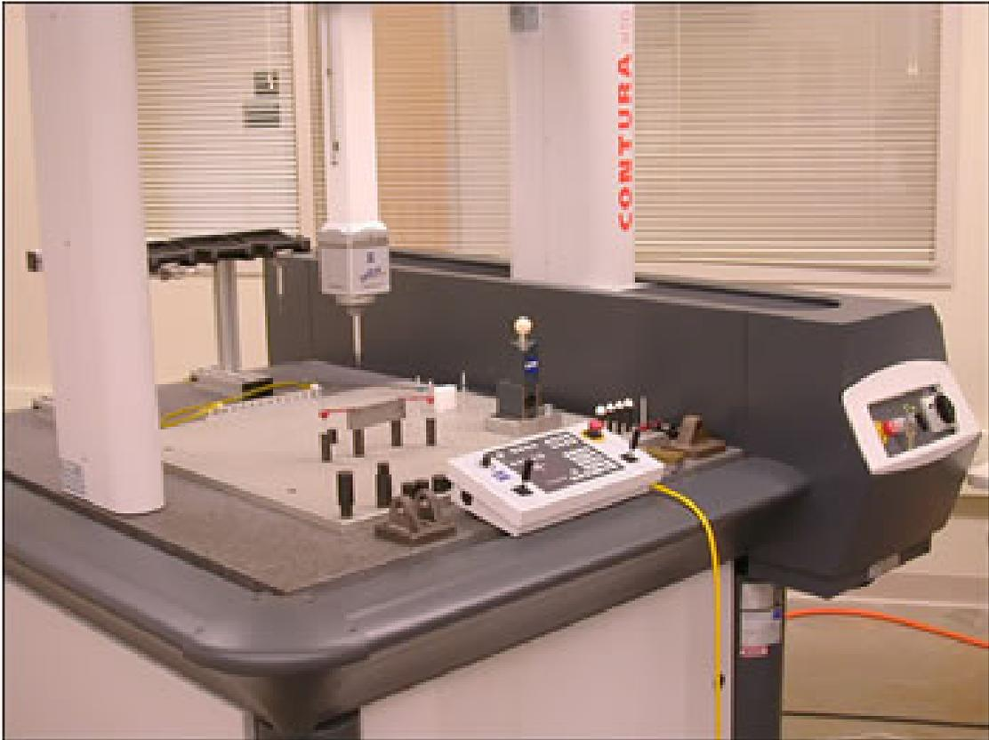
*Figure 2.1:* Coordinate Measuring Machine.
