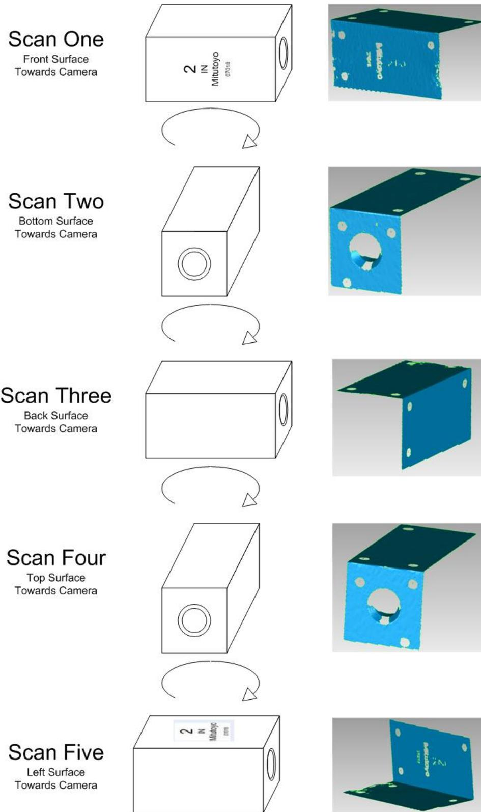
*Figure 3.8: Gage block orientation for each scan (left) and local point clouds of the five corresponding scans (right).*
