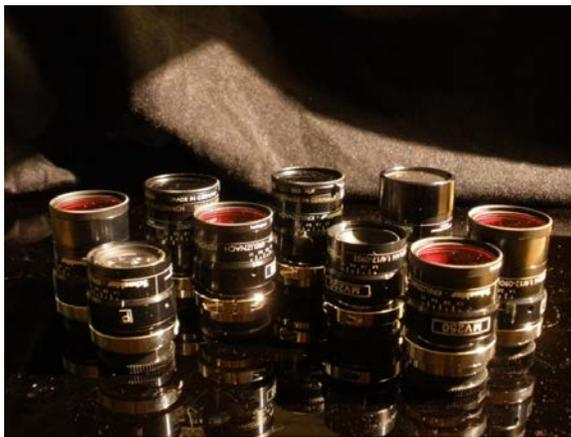
*Figure 3.1:* The lenses for the 90mm, 500mm, and 250mm for the projector and left and right camera
