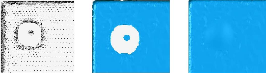
*Figure 2.12: Measured point cloud around a reference point. Image created using scan data from a 1" gage block acquired using the ATOS system*
