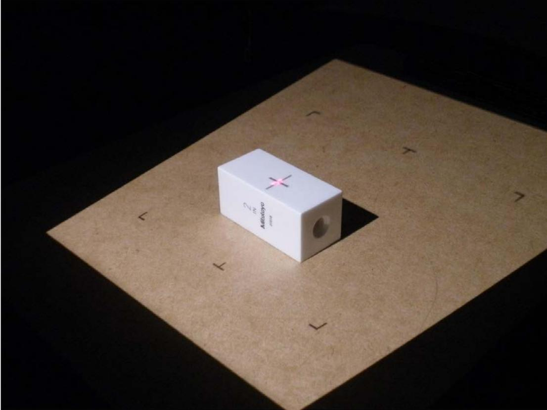
*Figure 3.7:* Two inch gage block inside the 120mm measurement volume.
