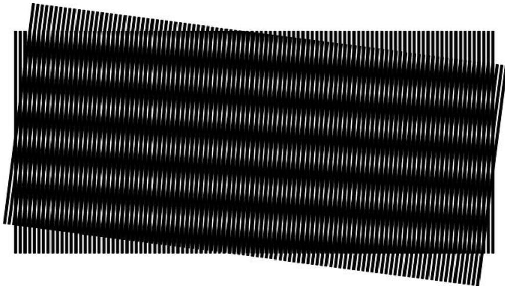
*Figure 2.5:* Moiré pattern of two identical line patterns superimposed at an angle on a flat surface. Adapted from “Moire Metrology,” by Jin, L. (2003). In T. Yoshuzawa (ed.), *Handbook of Optical Metrology Principles and Applications* (pp. 263-280). Boca Raton, FL.: CRC Press.
