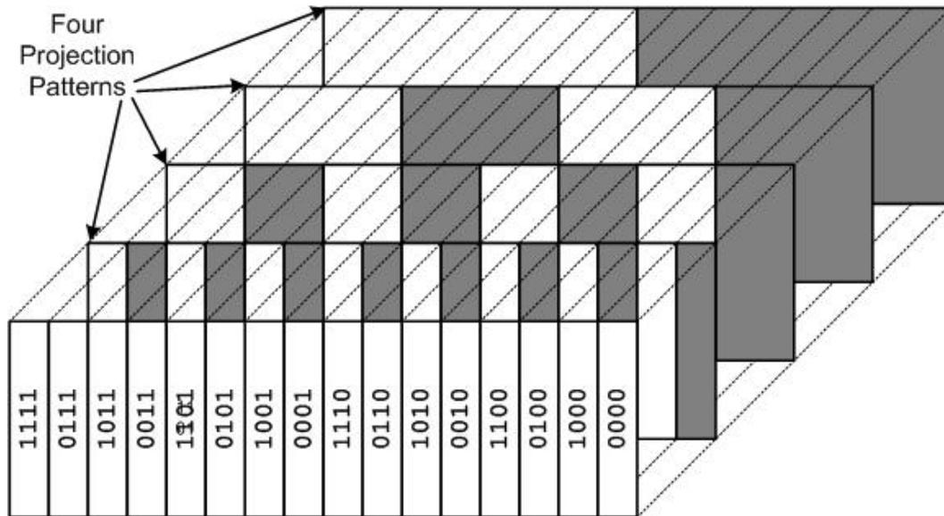
Figure 2.9: Gray code using four projection patterns. Adapted from “Photogrammetric Matching of Point Clouds for 3D-Measurement of Complex Objects,” by Reich, C. (1998). *SPIE*, 3520, 100-110
