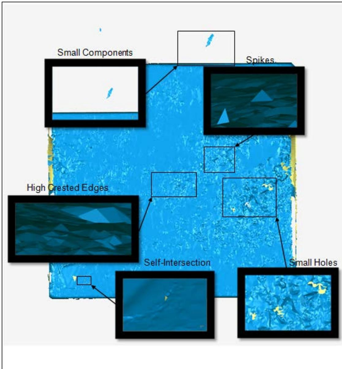
*Figure 2.15:* Polygon mesh abnormalities. Image created using scan data from a 1" gage block acquired using the ATOS system.
