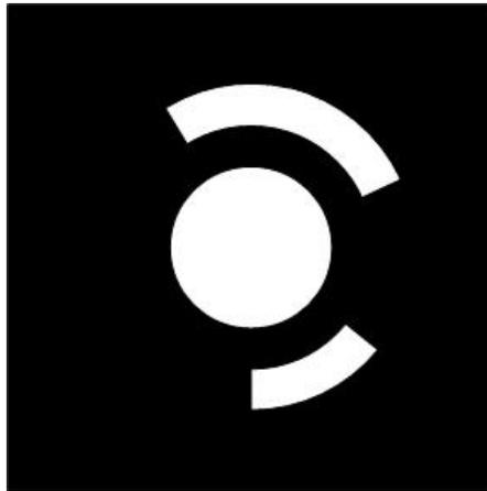
*Figure 2.4:* Coded target based from observed close range photogrammetry targets.
