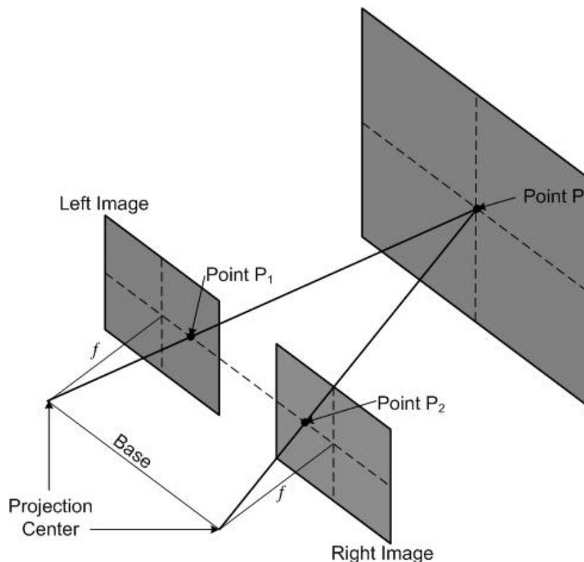
*Figure 2.3:* Diagram of photogrammetry center of projection principle. Adapted from “Photogrammetry,” by Kochi, N. (2003). In T. Yoshuzawa (ed.), *Handbook of Optical Metrology Principles and Applications* (pp. 511-529). Boca Raton, FL.: CRC Press.
