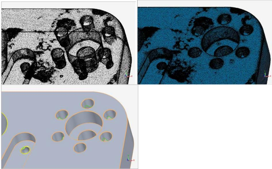
*Figure 2.14:* Transformation of a point cloud into a parametric solid model. Image created using scan data from an object acquired using the ATOS system.
