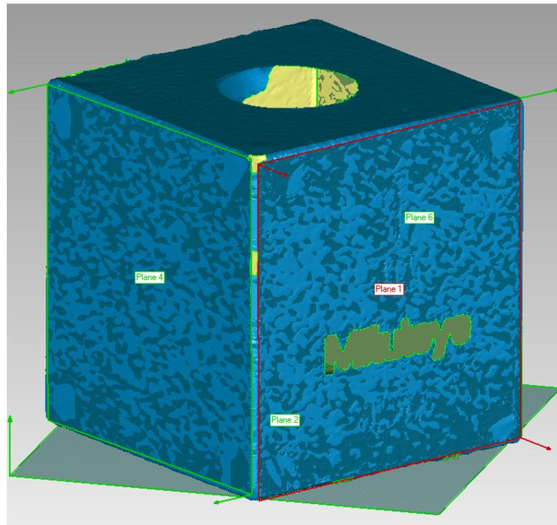
*Figure 3.10:* Three planes used to locate the CAD data in 3D space, image created using scan data from a 1" gage block acquired using the ATOS system
