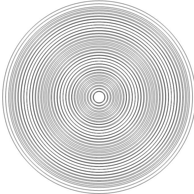
*Figure 2.6: Out-of-plane moiré pattern. Adapted from “Moire Metrology,” by Jin, L. (2003). In T. Yoshuzawa (ed.), Handbook of Optical Metrology Principles and Applications (pp. 263-280). Boca Raton, FL.: CRC Press.*
