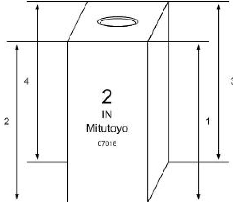
*Figure 3.14:* Position of the four measurements taken from gage block scan data.
