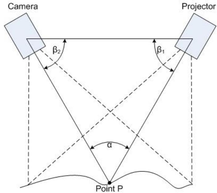
*Figure 2.7:* Distortion of coded light when projected onto an object. Image was taken using the ATOS white light scanner.
