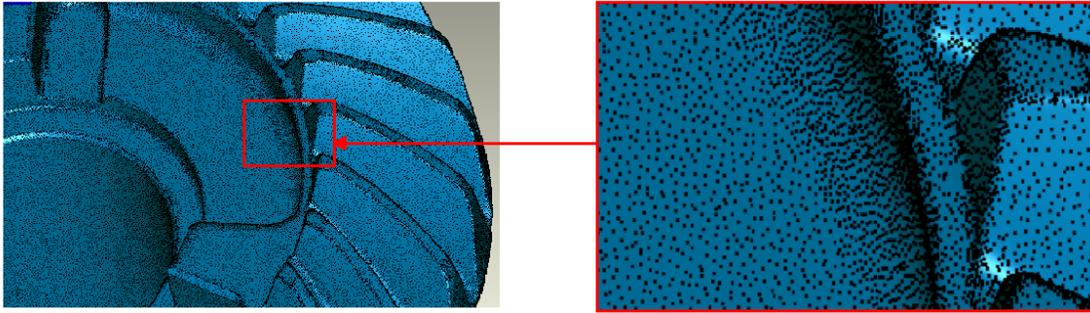
*Figure 3.9:* Change in point density in curved regions. Image created using scan data from a gear acquired using the ATOS system.
