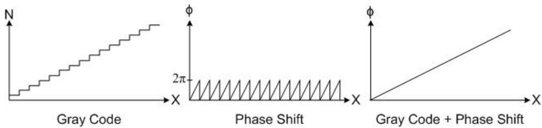
Figure 2.10: Gray code + phase shift. Adapted from “New Approach for Automatic Surface Reconstruction with Coded Light,” by Bergmann, D. (1995). *SPIE*, 2572, 2-9
