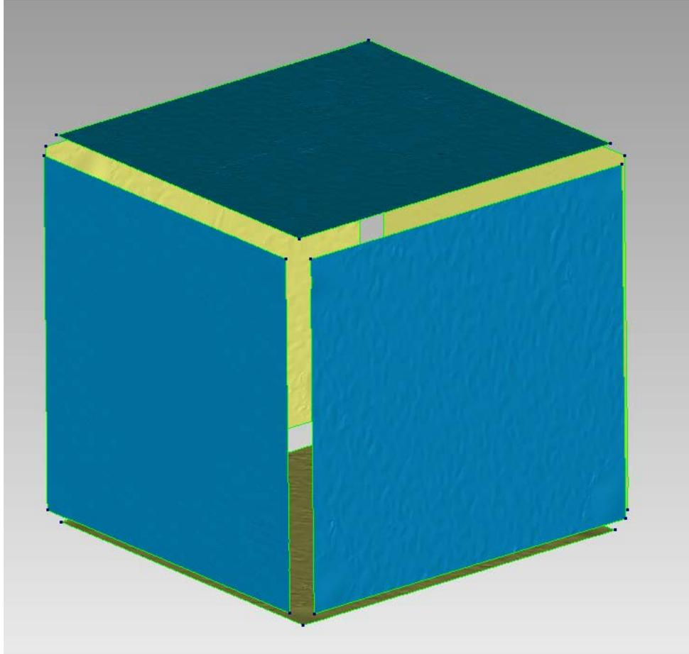
*Figure 3.12:* Polygon mesh after data were removed from the edges, image created using scan data from a 1" gage block acquired using the ATOS system.
