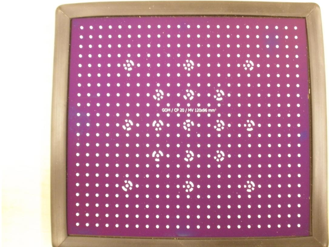
*Figure 2.13:* Calibration object for the 120mm measurement volume.
