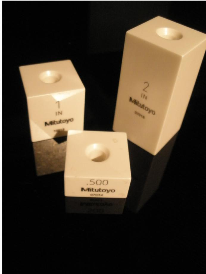
*Figure 3.4:* Mitutoyo ceramic square gage blocks, sizes 1 inch, 0.5 inch, and 2 inch, certified by NIST used during data collection.
