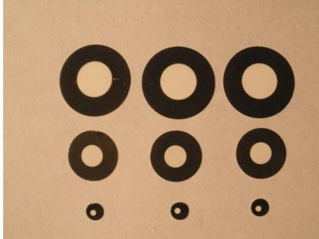
*Figure 2.11:* Reference points, 5mm on top, 3mm in the middle, and 0.8mm on the bottom
