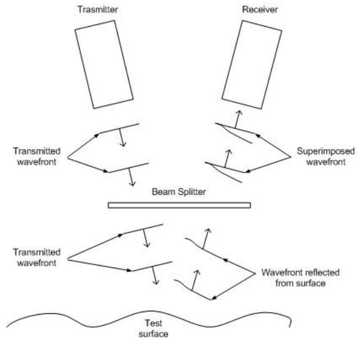
*Figure 2.2: Simple diagram for interferometry. Adapted from “Interferometry” by Page, D. (2003). In T. Yoshuzawa (ed.), Handbook of Optical Metrology Principles and Applications (pp. 191-217). Boca Raton, FL.: CRC Press.*
