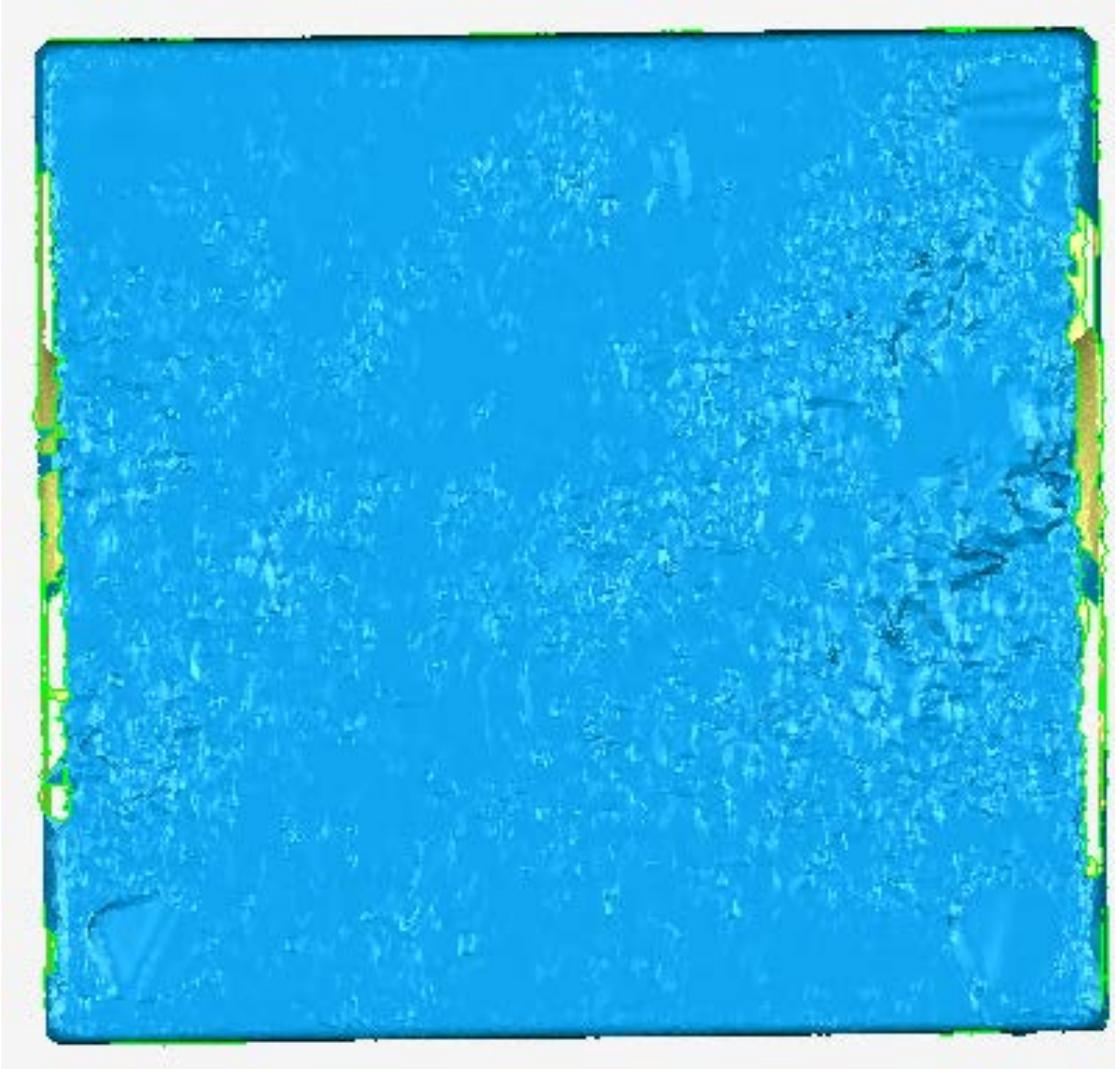
*Figure 2.16:* Repaired polygon mesh. Image created using scan data from a 1” gage block acquired using the ATOS system
