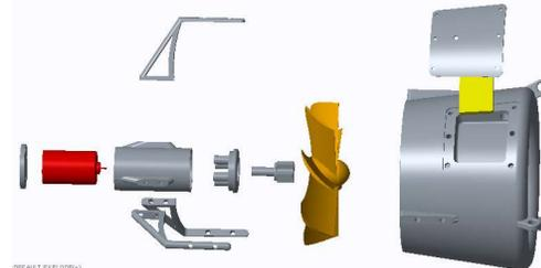
The figure above is a disassembled view of the final product in which had a low reproduction cost due to the utilization of 3D printing most of the parts. These parts were printed using ABS to ensure that they would not degrade and pollute the water source while the PHG is being used.
