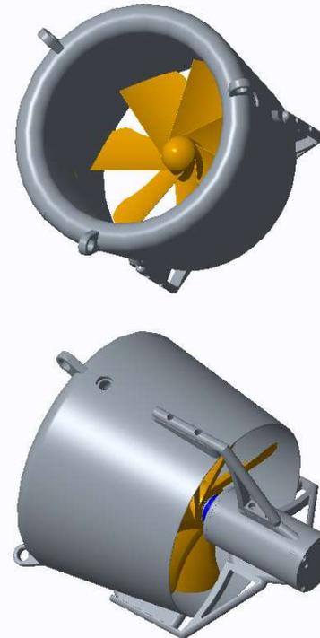
The figures above are two auto-CAD generated views of the assembled Portable Hydro-electric Generator.
