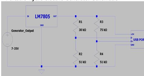
The figure above shows the circuitry inside the PHG going from the generator output to the USB port. The LM7805 was used to regulate the voltage and restrict it to a constant 5 Volts. The following four resistors are used to enable the fast charging setting within smart phones by connecting to the data inputs (D+ and D-) to allow for smartphones to receive more than only 0.5 A which it is restricted to if these voltages differ too far from these fast charging voltages.
