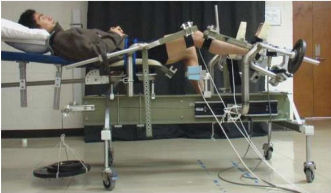
**Figure 1.** The Vermont knee laxity device.
