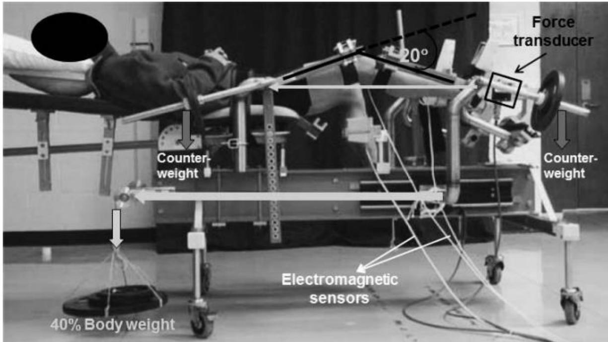
Figure 1. The Vermont Knee Laxity Device.
