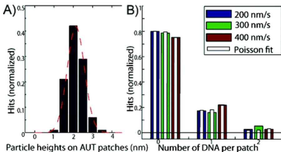
**Figure 3.** (A) Histogram of the heights of 100 rod-like particles observed on AUT patches, with Gaussian fit.  $\mu = 2.13 \text{ nm}$ ,  $\sigma = 0.44 \text{ nm}$ . (B) Histogram of the number of DNA molecules per AUT patch as a function of write speed. Number of DNA per patch follows a Poisson distribution.
