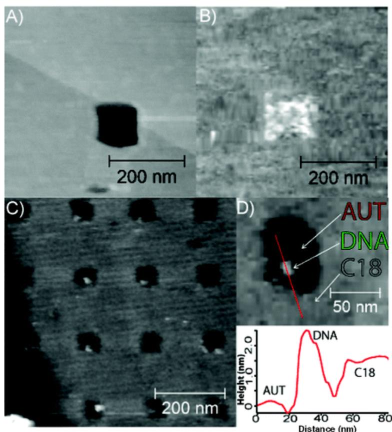
**Figure 2.** (A–C) Representative images of patches nanografted in solutions containing (A) 1  $\mu$ M DNA-SH in 1X TAE, (B) 1  $\mu$ M DNA-SH and 20  $\mu$ M AUT in 1X TAE, and (C)  $\sim$ 3 nM DNA-SH and 10  $\mu$ M AUT in 0.01X TAE. Individually resolvable DNA molecules are observed within an array of 50 nm  $\times$  50 nm AUT patches by tapping-mode AFM. (D) Single, patterned DNA molecule and height cross-section.
