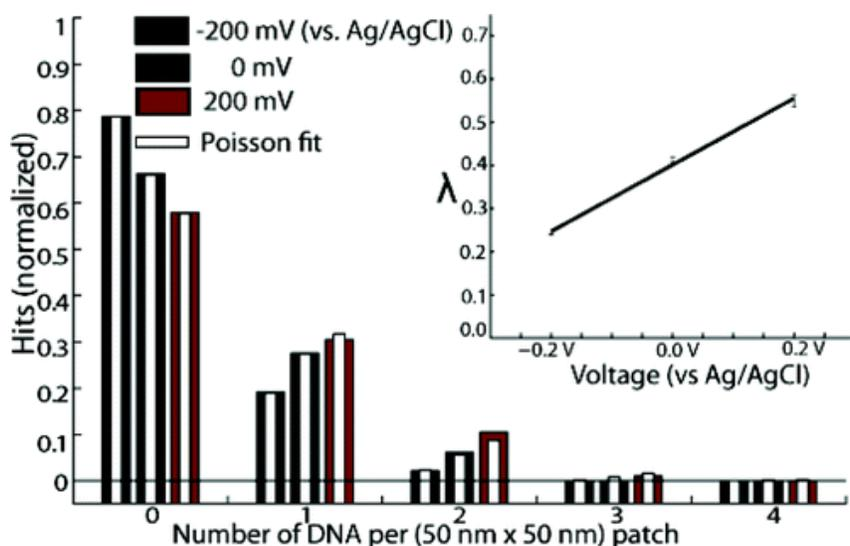
**Figure 4.** Experimental effects of applied potential during nanografting. Applied negative potential (black) during nanografting results in an increase in DNA squares with no DNA molecules, while application of a positive potential (red) results in an increase of patches with DNA. (Inset) Expected number of DNA per patch ( $\lambda$ ) as a function of applied voltage. Error bars were determined by uncertainty of the Poisson fit.
