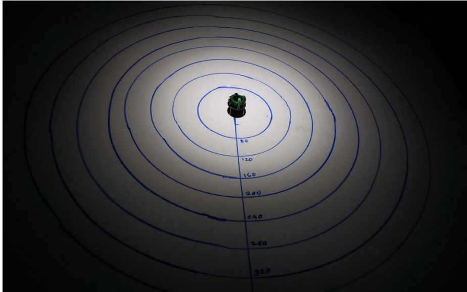
Figure 36. Small distance light sensitivity test for adding the second sensor
