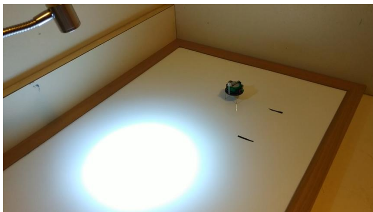
Figure 34. Move away from light test using new Kilobot (Moving Away)
