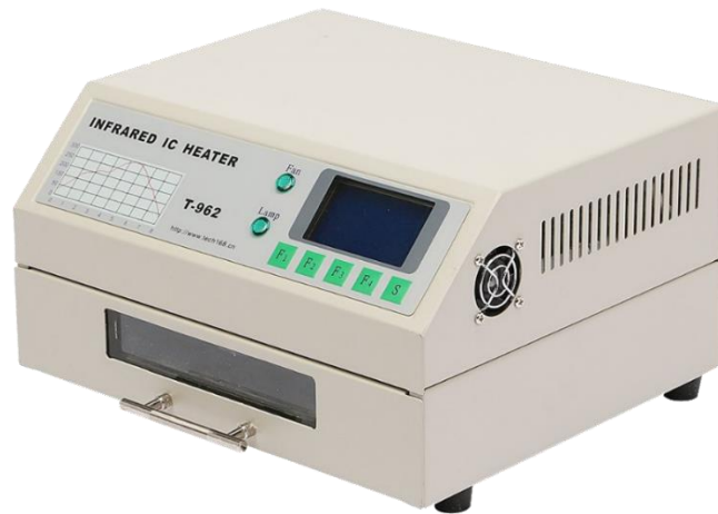
Figure 14. The reflow oven we used
