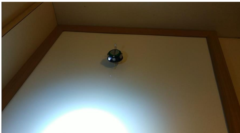
Figure 31. Move away from light test using old Kilobot (Stopped due to saturation)
