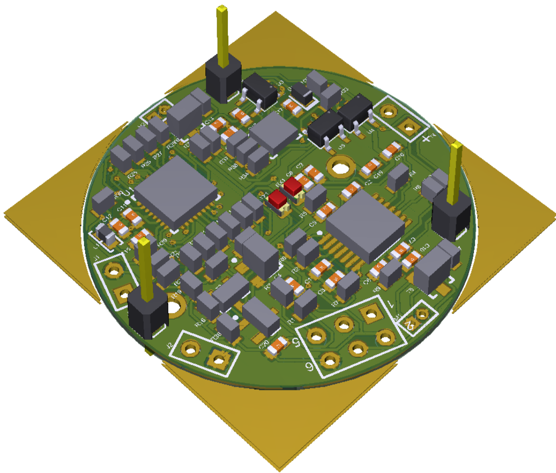
Figure 28. 3D view of PCB layout of Kilobot version 1.2
