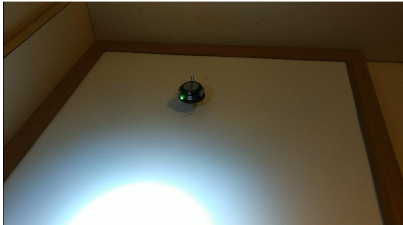
Figure 30. Move away from light test using old Kilobot (Starting)
