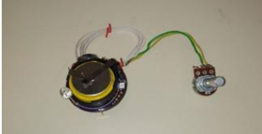
Figure 21. Kilobot with a potentiometer for ambient light test
