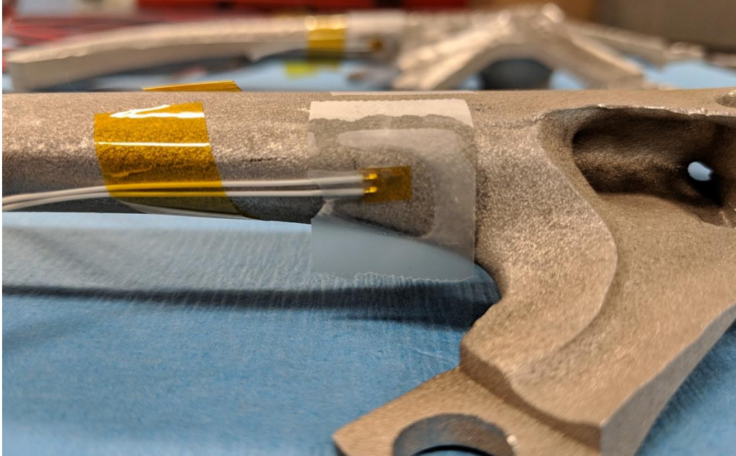
Figure 3.64: Strain Gauge on the Optimized Crank Arm
