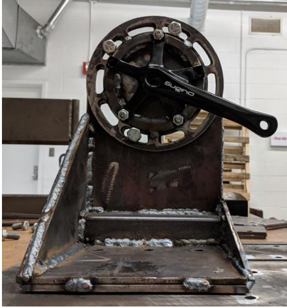
Figure 3.57: Front View of Assembled Structure
