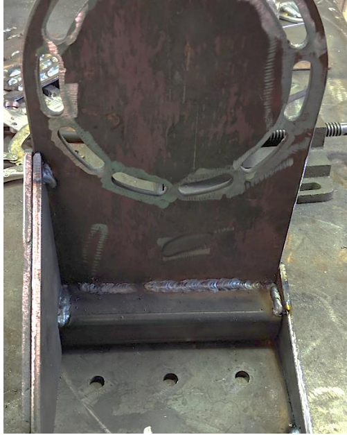
Figure 3.55: Square Tubing Assembly
