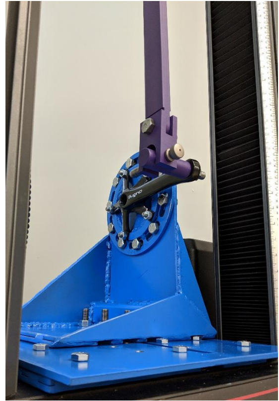
Figure 4.39: Side View of Testing Apparatus Mounted in the Instron Tensile Tester
