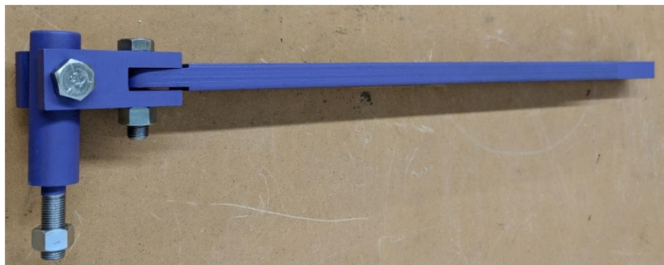
Figure 4.37: Finalized Pedal Assembly
