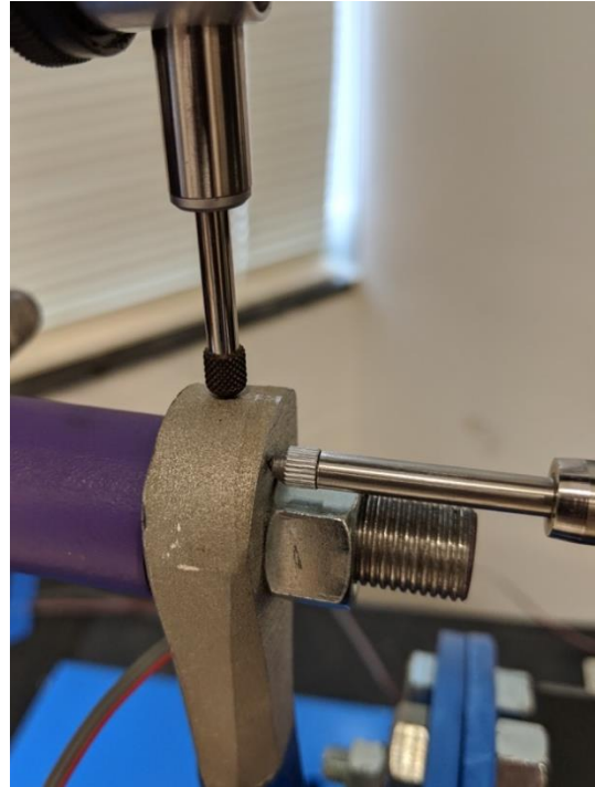
Figure 3.68: Dial Indicator Alignment
