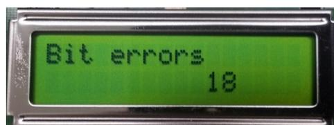
Figure 19: Display of 18 Errors on Modified Fiber Optic Transceiver Design.
