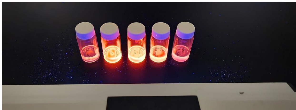
Figure 46. TTA-coated Eu:CaF 2 nanoparticles under a low power and low-cost benchtop UV lamp (365nm). The nanoparticles show a bright red emission.
