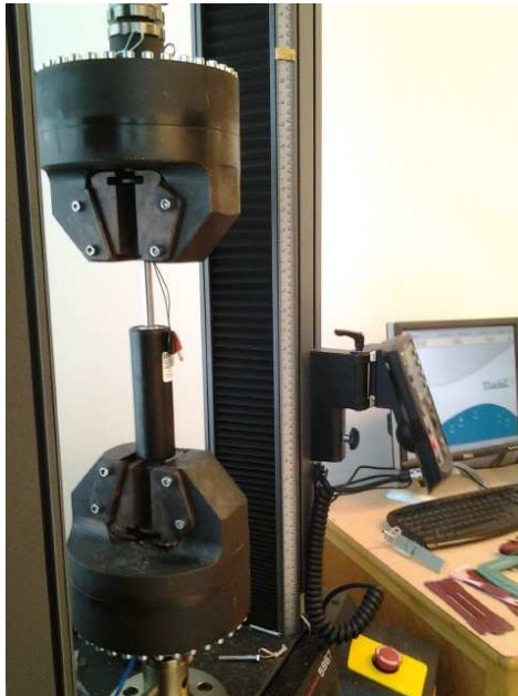
Figure 4.2: Test setup for damper characterization.
