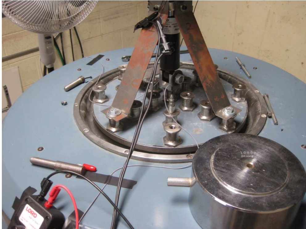
Figure 4.8: Damper support fixture – complete assembly.
