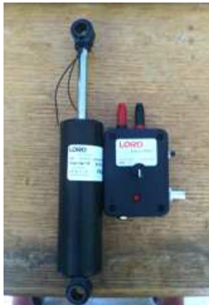
Figure 4.1: MR Damper and Control Kit.
