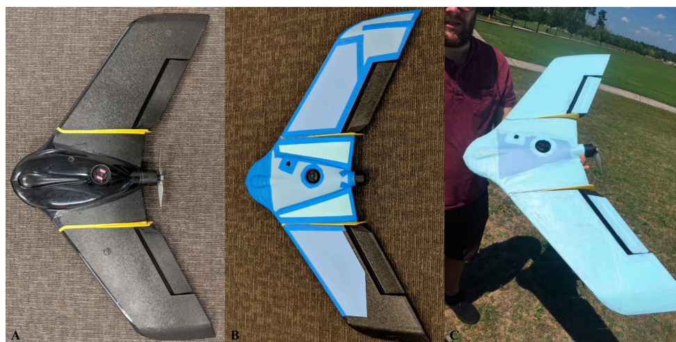
Figure 3. senseFly eBee Plus fixed-wing drone. (A) Flight 1—No modifications. (B) Flight 2—dazle camouflage. (C) Flights 3 through 5—solid sky-blue camouflage.
