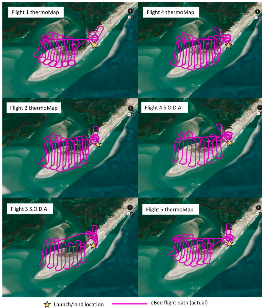
Figure 2. Flight missions using the senseFly eBee plus equipped with thermoMap or S.O.D.A. sensors on Lea-Hutaff Island. See Table 1 for additional mission parameter information. S.O.D.A flights use the same flight block. Thermal flights 2–4 used the same flight block, and thermal flight 3 is not shown in the figure.
