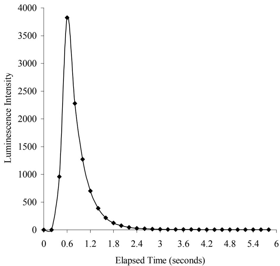
Figure 1: Continuous data stream of luminescence intensity used to determine time interval on chemiluminescence instrument
