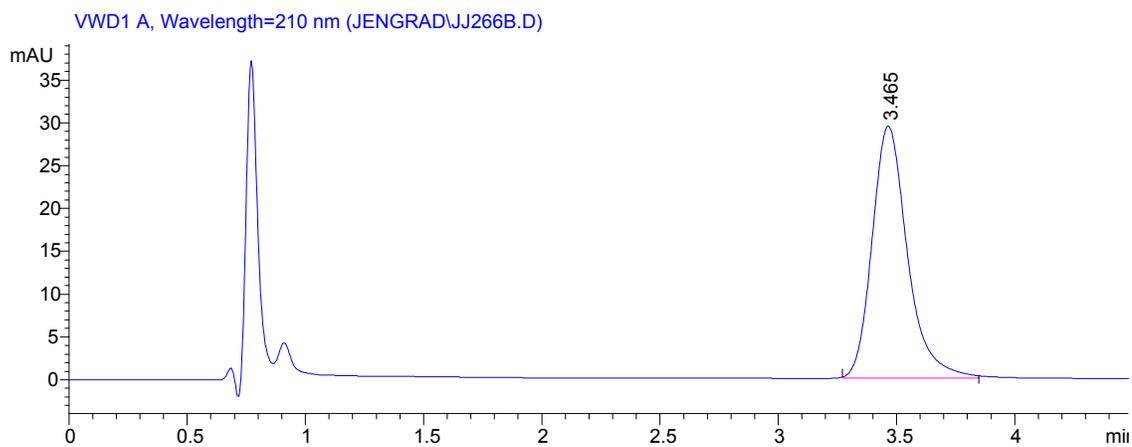
Figure 6: An HPLC chromatogram of DMH peak. The column: Hypersil Hypercarb, 50 x 4.6 mm I.D., 5-micron particle size; mobile phase: 0.10 M KCl solution mixed in ratio (97:3) with methanol; flow rate: 1.0 mL/ min, column temperature at 23°C; sample injection volume: 10  $\mu$ L, and UV lamp: 210 nm.
