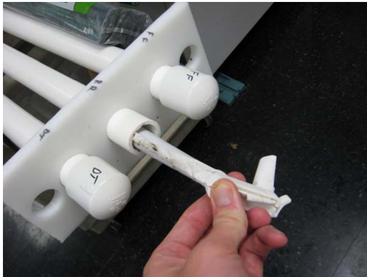
Figure 7: Sediment in membrane packet being inserted into SEM
