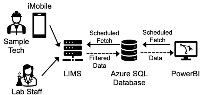
Fig. 1. Diagram depicting data flow from field to dashboard.
