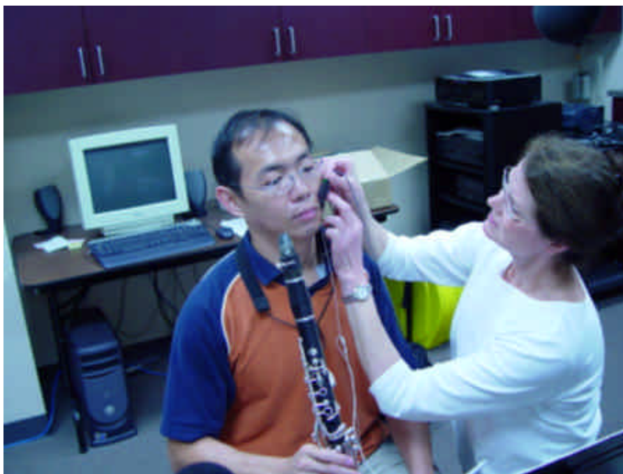
Figure 9. Dr. Evelyn Davis Attaches the Surface Electrodes to the Zygomaticus Major and the Reference Electrode is Visible on the Player's Left Median Clavicle
