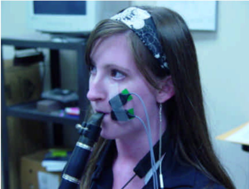
Figure 8. Left-Side Facial Electrode Placements
