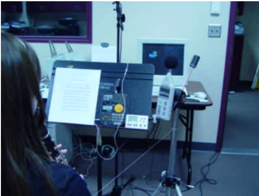
Figure 6. View of Instrumentation from behind Clarinetist, Showing (Left to Right) the Metronome and Tuner on the Music Stand and the Sound Pressure Meter to the Right
