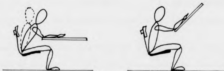
Figure 1.--Angle of Body Bend Decreases as Tilt of Drafting Surface Increases
