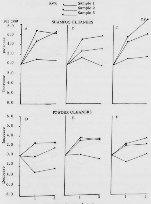
CHANGE IN PILE HEIGHT OF NYLON CARPETS AFTER CLEANING
