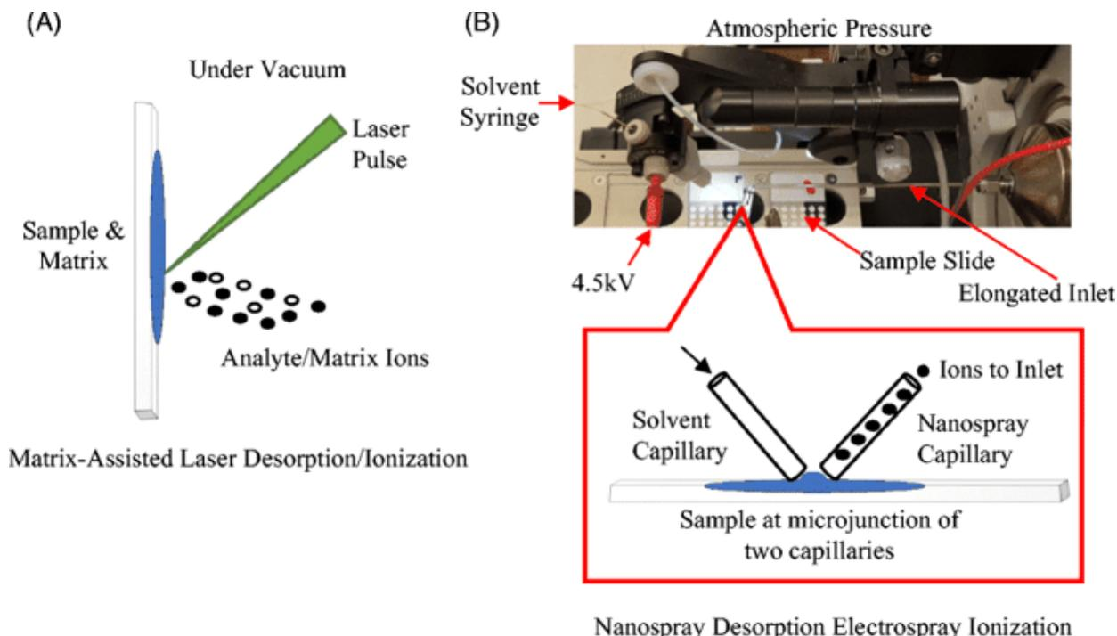
**Fig. 1.** Schematic diagram of (A) matrix-assisted laser desorption/ionization (MALDI) and (B) nanospray desorption electrospray ionization. A 2–4  $\mu\text{L}$  sample was air-dried on a glass slide. Fused silica capillary with 49  $\mu\text{m}$  internal diameter was  $\sim 1\text{--}2$  mm above the sample, and the flow rate of solvent was 3.5  $\mu\text{L}/\text{min}$
