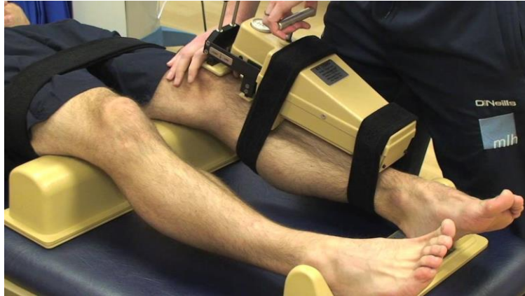
Figure 3.1. Experimental Set-Up and Participant Positioning for the Anterior Knee Laxity (AKL) Assessment.
