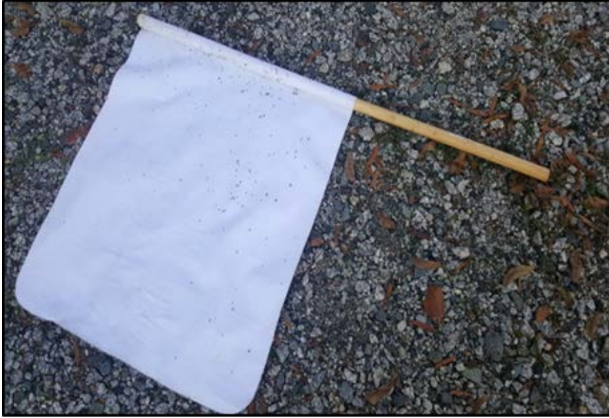
Figure 2.1. Tick Collection Flag. The flag was constructed using a .03 m by 1.22 m wooden dowel, with a 1 m 2 flannel sheet attached to the dowel using heavy gauge staples
