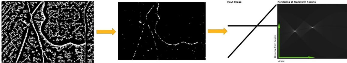
Figure 4.8. from [109], Automatic Line recognition using Hough Transformation. Left Ridge filter is applied by convolving Hessian Matrix and extracting eigen values. (center) Image erosion to remove noise. (right) example of a simple Hough Transformation from 2 lines to two points.
