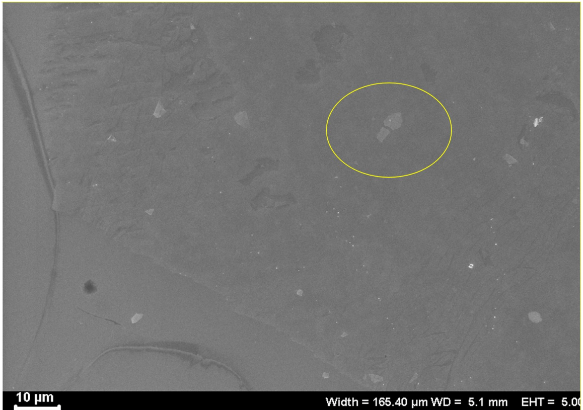
Figure 4.14. NbSe 2 flakes on SiO 2 covered by graphene.
