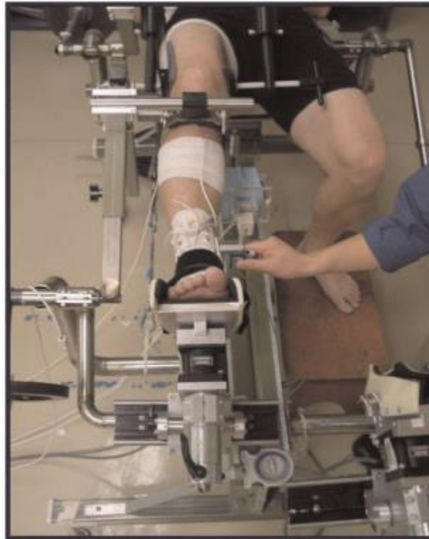
Figure 2. A handheld force transducer applied resistance to the medial and lateral aspect of the distal tibia to create a 10 Nm varus and valgus torque at the knee.
