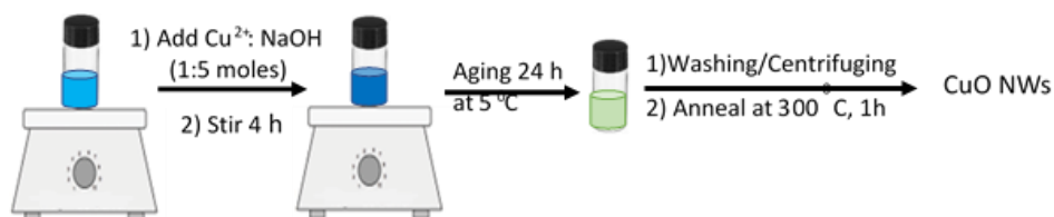
Figure 10: Experimental Setup of Fabrication of Cu(OH) 2 /CuO NWs
