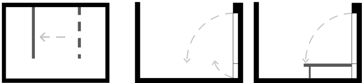
Figure 54. Convertible Furniture and Spaces Diagram Illustrating How Sliding Partitions and Pullout Furniture Transform a Space
