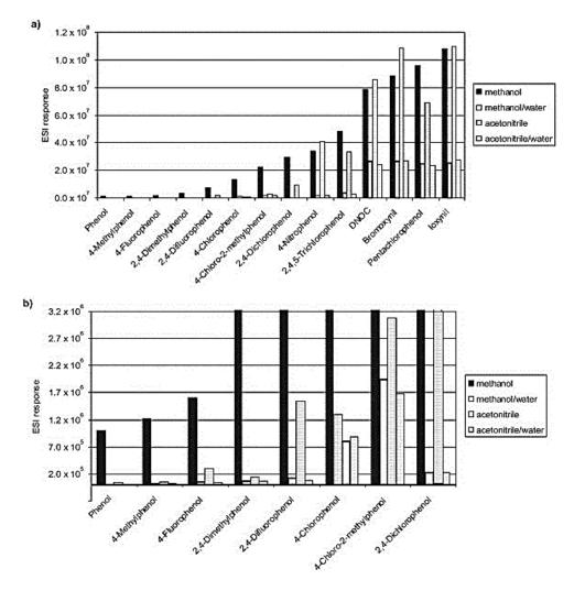
**Figure 3.** (a) ESI response of all of the phenolic compounds from Table 1 compared in various solvents. The analytes have highest response in neat methanol. The addition of water to the solvents causes a decrease in response of all analytes. Response in methanol:water (1:1) and acetonitrile:water (1:1) mixtures is similar. (b) An expanded view of the results for the less responsive analytes from Part **a**.
