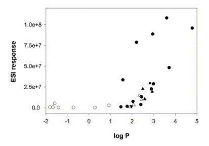
**Figure 2.** ESI response in methanol as function of analyte log P. (filled circle) Phenols, (open triangle) benzoic acids, (filled triangle) phenoxyalkanoic acids, (open circle) triazines. Response is positively correlated with log P for analytes having log P > 1.5. The four analytes that deviate by a higher response are p-nitrophenol, DNOC, bromoxynil and ioxynil (left to right).
