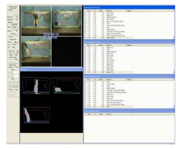
Figure 6-1. **HomeCage Scan**- HomeCage Scan (Clever Systems, Inc) measuring cage activity for each cage. Real-time behaviors are quantified by determining anatomical features of each rat and the location of food and water source to identify behavior.
