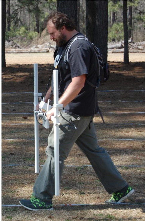
Figure 10. Bartington 601 Dual Magnetic Gradiometer
