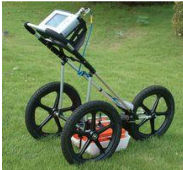
Figure 11. GSSI 3000 Ground-Penetrating Radar (GPR) with a 400 MHz Antenna
