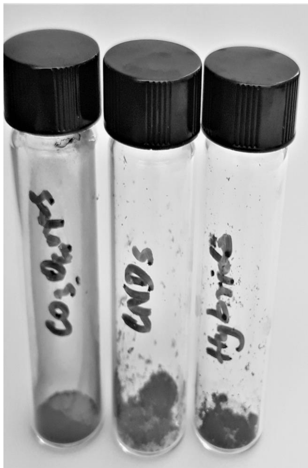
Figure S2.2. Texture of the synthesized \text{Co}_3\text{O}_4 , CNDs, and \text{Co}_3\text{O}_4 @CNDs hybrid NPs
