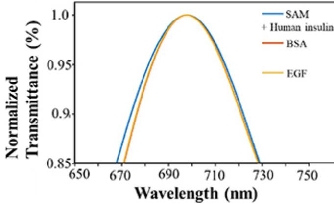
**Figure 6.** Measured peak shift for BSA and EGF to test the specificity of the plasmonic nanoledge device.
