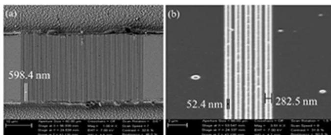
**Figure 3.** (a) SEM image of nanoledge array with 600 nm of periodicity. (b) Represent the FIB images of the nanoledge.
