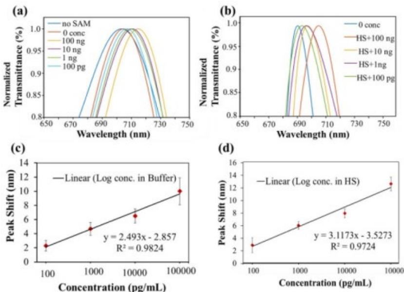
**Figure 5.** Representation of peak shift for anti-insulin antibody (a) in buffer and (b) in human serum; (c) and (d) show correlation of concentration of anti-insulin antibody with respect to wavelength peak shift, the straight line shows the linear fit.
