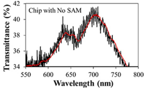
**Figure 4.** Represents the transmittance curve (smoothed in red color and, unsmoothed in black color) of fabricated plasmonic chip without any modification.
