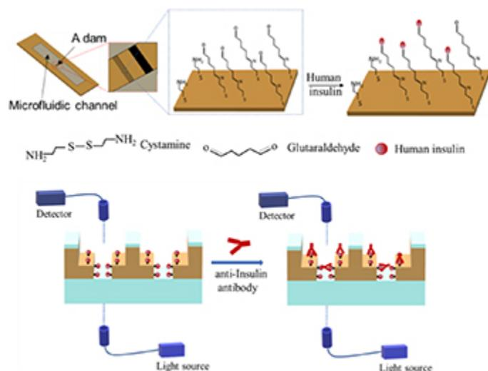
**Figure 1.** Illustration of the gold surface functionalization at the gold surfaces of the nanoledge array to immobilize human insulins and the model of plasmonic nanoledge device used for biomarker or biomolecule detection.
