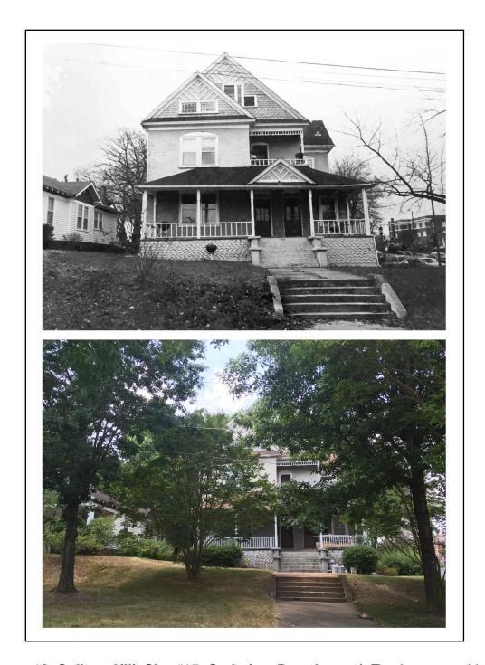
**Figure 10. College Hill, Site #15, Coded as Deteriorated.** Top image, archival photograph. Bottom image, photograph taken Summer 2015. Field notes: Jackson street. Replacement windows. Structure needs paint. Balustrade at top falling off. Shingles missing. Deteriorating. See Appendix F for supplemental photograph to support field notes.
