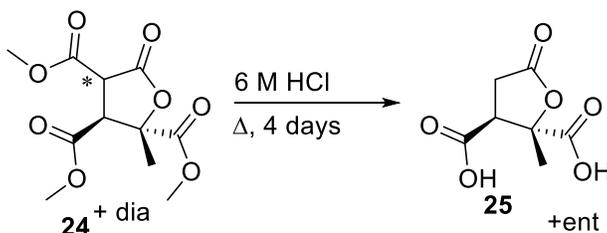
The crude produce **24** (0.2202 g, 1eq) was refluxed in 6 M HCl (4.5 mL) for 4 days followed by the removal of solvent by reduced pressure. The concentrated reaction was dissolved three time in 20 mL of water and evaporated each times to removes residual HCl. The brown oil was dissolved in 20 mL of water and treated with activated charcoal for 30 minutes at 80 °C. The reaction was filtered through a 1 cm bed of celite to remove the charcoal. The solvent was removed with reduced pressure.
