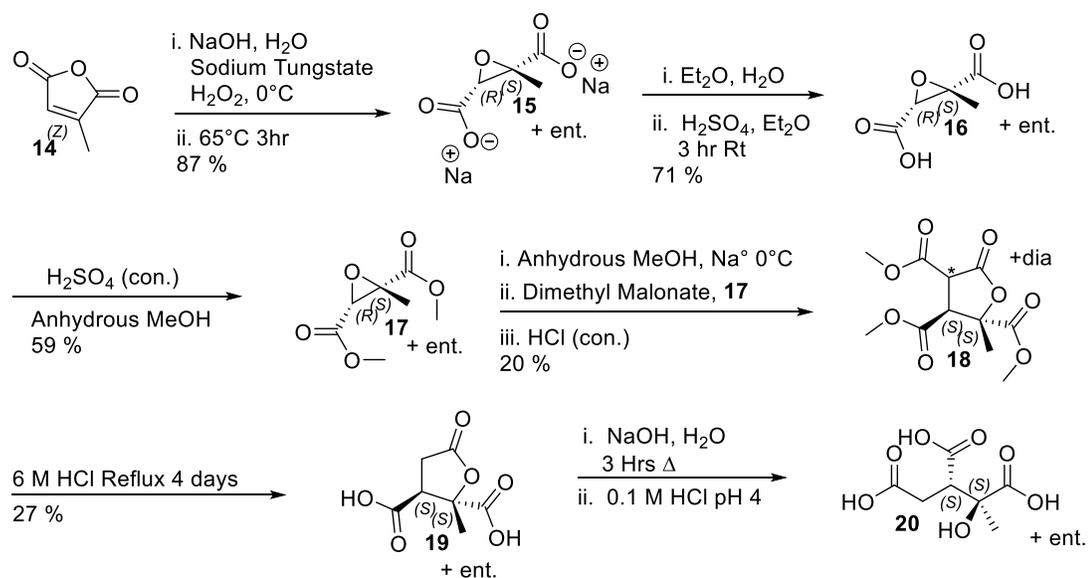
The published literature procedures by Brock et al. had to be modified greatly in order for the reactions to be reproducible for our lab. The esterification required two reagents to be distilled prior to the reaction. A previous graduate student decided to utilize a Fischer esterification<sup>36</sup> instead because only methanol would need to be distilled. The lactonization was altered by increasing the equivalents of sodium metal used to
