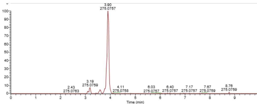
**Figure 16. Base Peak Chromatogram of 2-methyl-5-oxo-2,3,4-tricarbomethoxytetrahydrofuran.** The base peak chromatogram obtained from mass spectrum analysis shows two product peaks. This is due to three stereocenters formed during the reaction. There is due to diastereomer formation and 8 stereoisomers being present.
