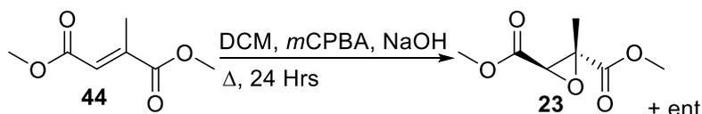
*meta*-Chloroperoxybenzoic acid (0.4923 g) was dissolved in dichloromethane (4.4 mL) and reacted with sodium hydroxide (0.1374 g). To the reaction dimethyl mesaconate (0.21 g) was added and refluxed for 24 hours. The solvent was removed with reduced pressure followed and the obtained white solid dissolved in saturated sodium
