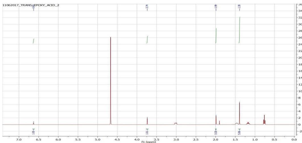
**Figure 17. <sup>1</sup>H NMR Analysis of Oxone Reaction.** The obtained <sup>1</sup>H NMR (D<sub>2</sub>O, 400 MHz) shows both starting material and the desired epoxide present. The mesaconic acid peaks appear at 3.63 and 1.99 ppm. *Trans*-epoxymethylsuccinic acid peak are located at 1.39 and 3.74 ppm.
