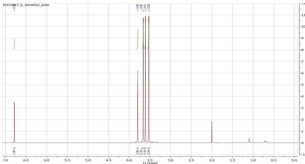
**Figure 20.  $^1\text{H}$  NMR of Trimethyl *E*-Aconitate.**  $^1\text{H}$  NMR was conducted to confirm the presence of the desired compound. The product peaks are observed at 3.53, 3.61, 3.66, 3.80, and 6.78 ppm.
