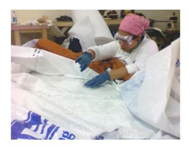
Figure 9. Stitching Together Layered Materials
