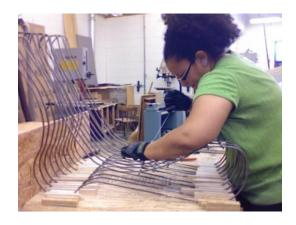
Figure 19. Tying Down Steel Cross Bars
