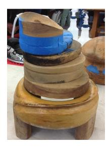
Figure 61. Stacking of Wood Block Forms
