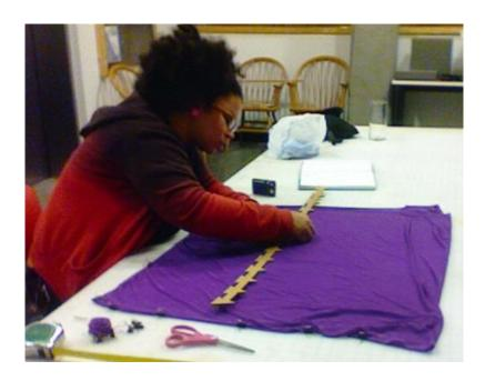
Figure 33. Laser Cut Cardboard Pattern Template
