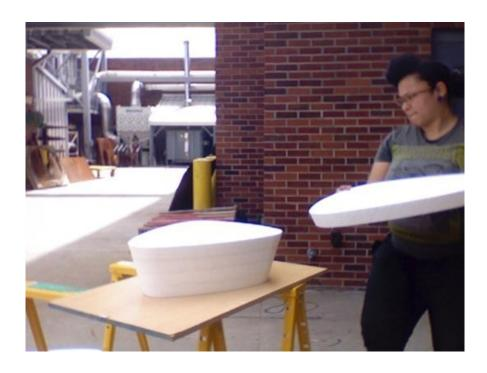
Figure 45. Gluing Foam Layers
