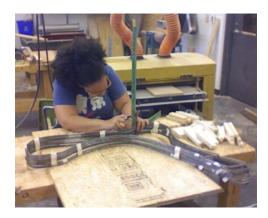
Figure 20. Marking Knot Location for Perpendicular Rods
