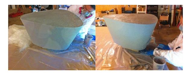
Figure 47. Rolling Fiberglass onto Surface
