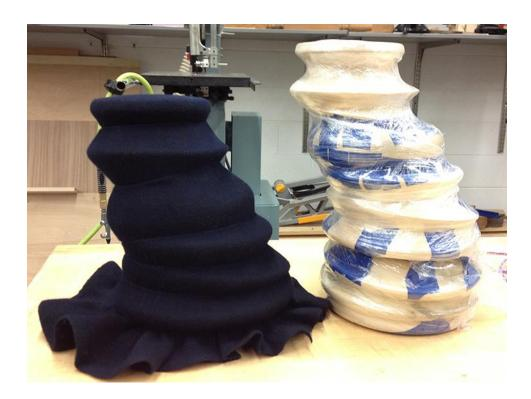
Figure 63. Custom Wood Form for Shaping Felt
