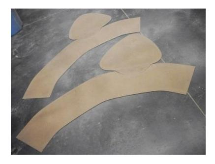
Figure 43. CNC Routed Templates
