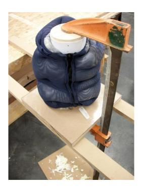
Figure 32. Foam Injection Around a Glass Vase
