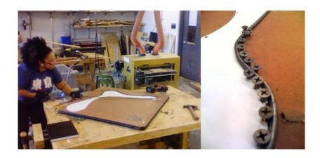
Figure 17. Bending Steel Rods
