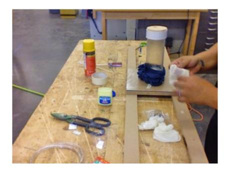
Figure 37. Textile Sac Slipped Over Glass Vessel
