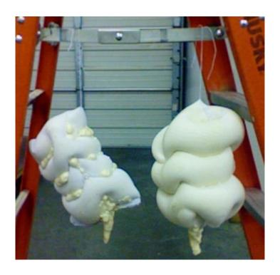
Figure 31. Foam Injection of Two Types of Fabrics
