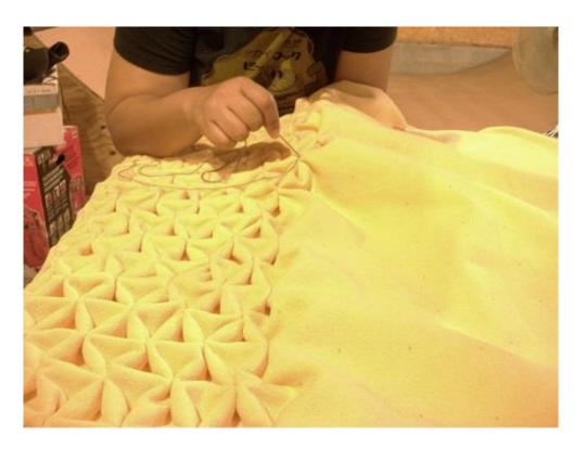
Figure 48. Sewing Honeycomb Technique
