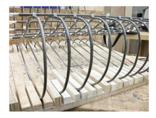
Figure 18. Slotted Platform System
