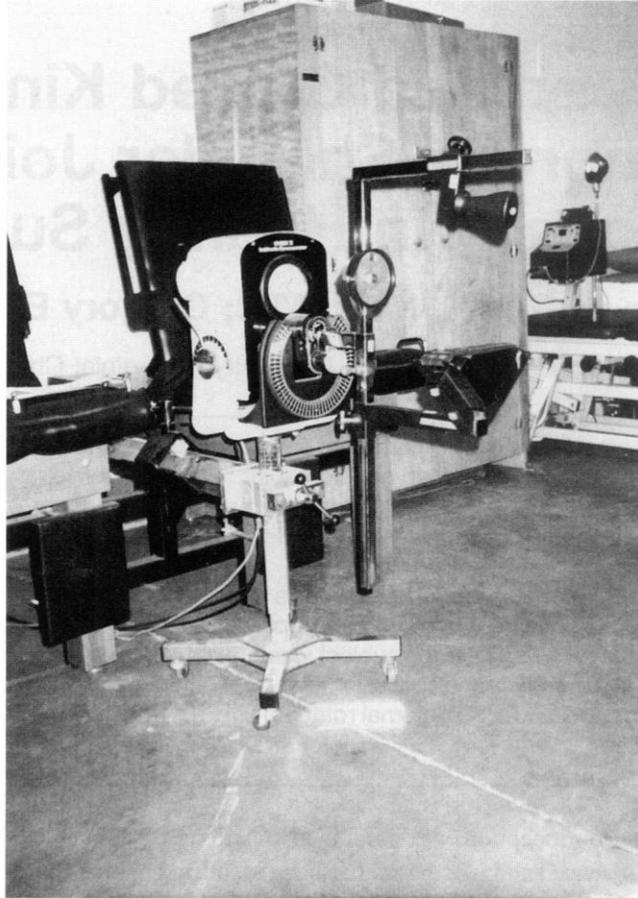
**Figure 1. A flexometer was attached to the arm of the Cybex to determine the angle of shoulder rotation.**
