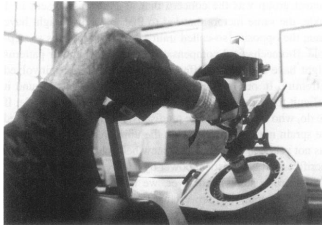
Subject positioned on the Kin Com 125 AP isokinetic dynamometer for eversion strength testing.
