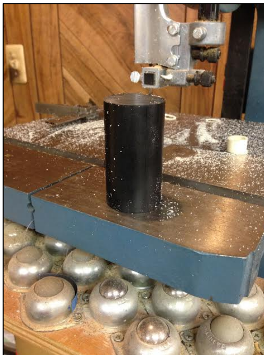
Figure 4. Delrin after Being Reduced to 3" in Length
