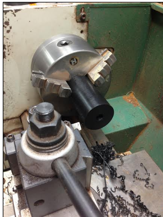
Figure 6. Picture of Barrel with Rough Bore.
