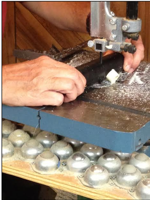
Figure 3. Delrin is Cut to 3" in Length.
