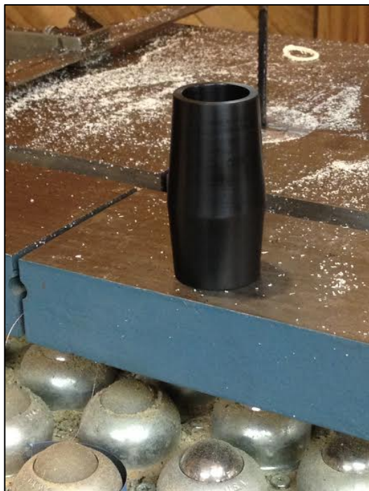
Figure 13. Finished Barrel after Receiving Final Bore Measurements.
