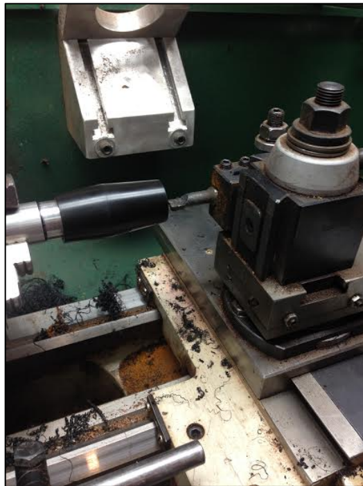
Figure 12. Barrel Receiving Final, Reverse-Taper Bore.
