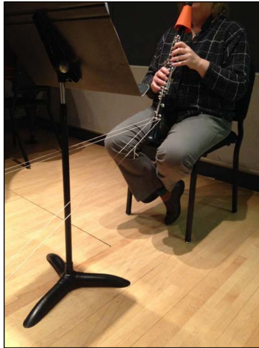
Figure 16. Player Setup Showing Triangulation.
