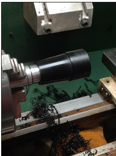
Figure 10. Barrel Being Prepared to Receive Exterior Contour and Mouthpiece Tenon Socket.
