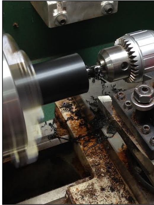
Figure 5. Delrin Receiving Rough Bore.
