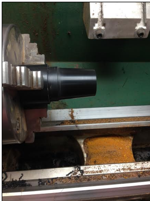
Figure 9. Barrel after Being Contoured
