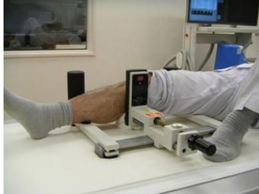
Figure II.8. TELOS Instrumented Knee Arthrometer [8]. To load the joint the black rotary handle extends the padded arm. Applied force is measured via sensors located within the extensible arm, while displacement is measured radiographically.
