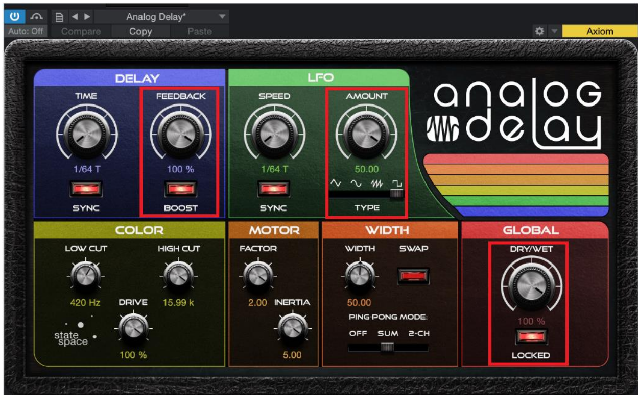
Figure 12. analog delay by state space set to self oscillate.
