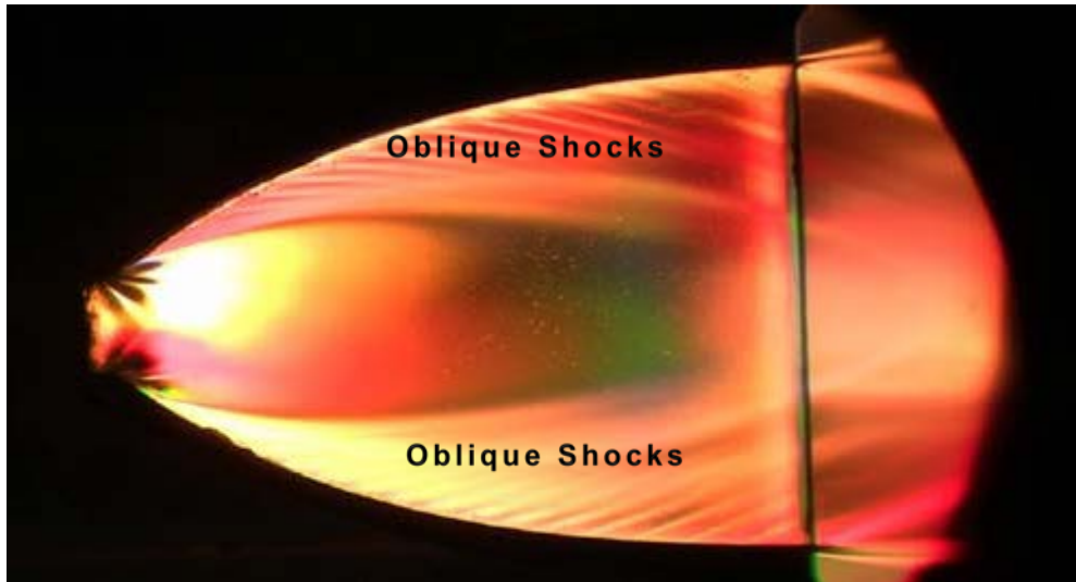
Figure 6-5: Schlieren image with oblique shocks
