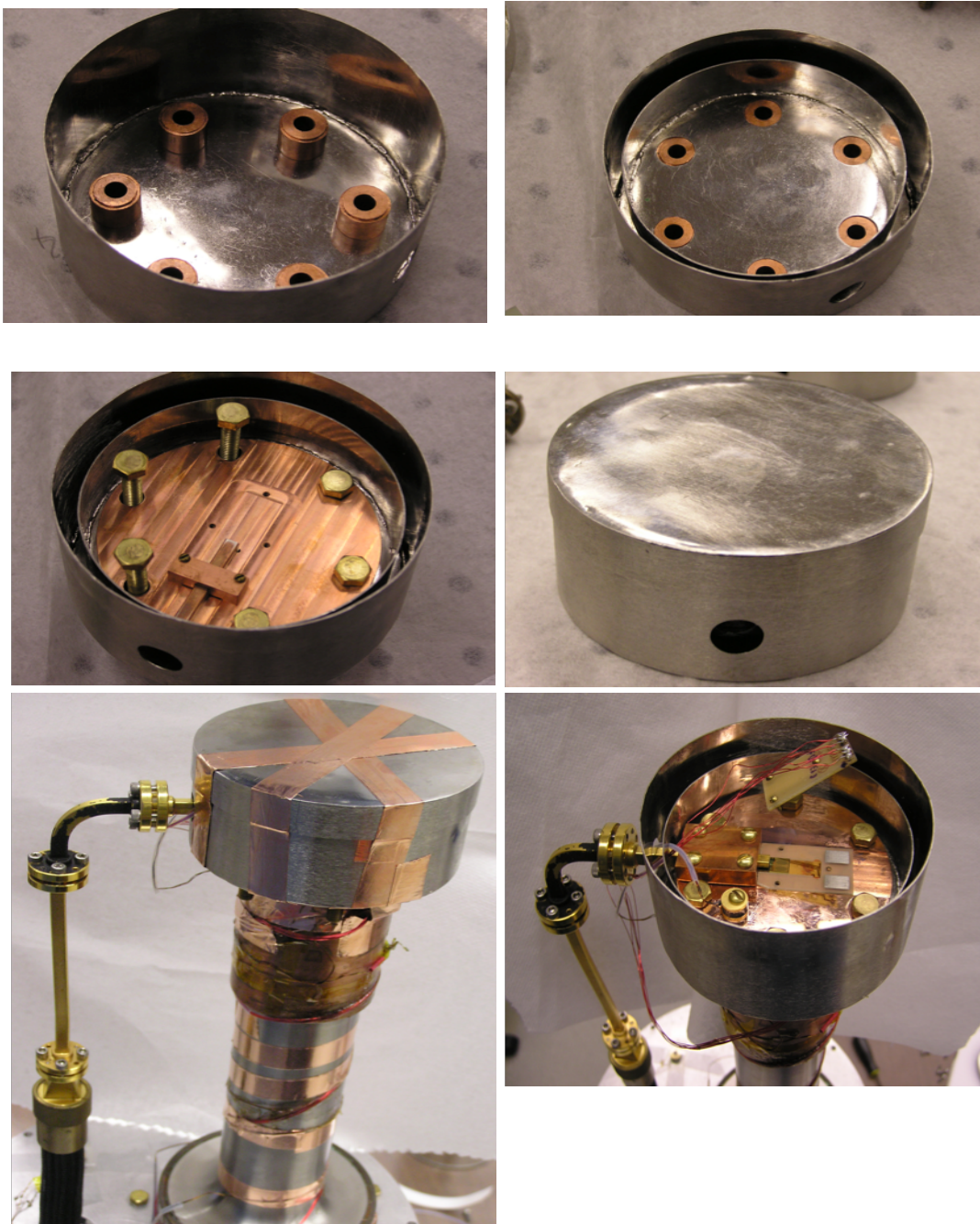
Figure 5.2: MuMetal ® magnetic shield enclosure for the JJA chip.
