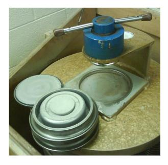
FIGURE 4-5: Rocklab ring grinder used in grinding the geopolymer concrete samples
