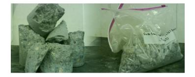
FIGURE 4-4: Crushed and size reduced geopolymer concrete sample
