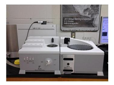
FIGURE 5-2: Laser diffraction particle size analyzer
