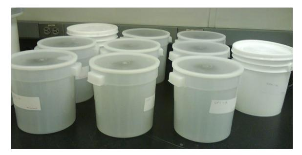
FIGURE 6-12: the tank leaching test setup
