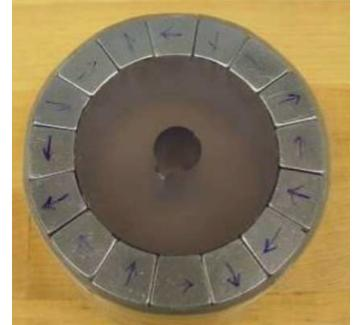
Figure 5.2: Picture of experimental four pole-pair EDW using 16 segmented NdFeB magnets [41].
