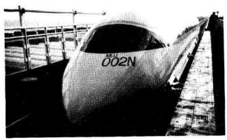
Figure 4.6: MLU002N test vehicle photo [14].
