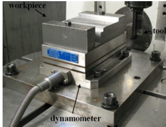
Figure 3.8: Experimental setup for milling force measurement.
