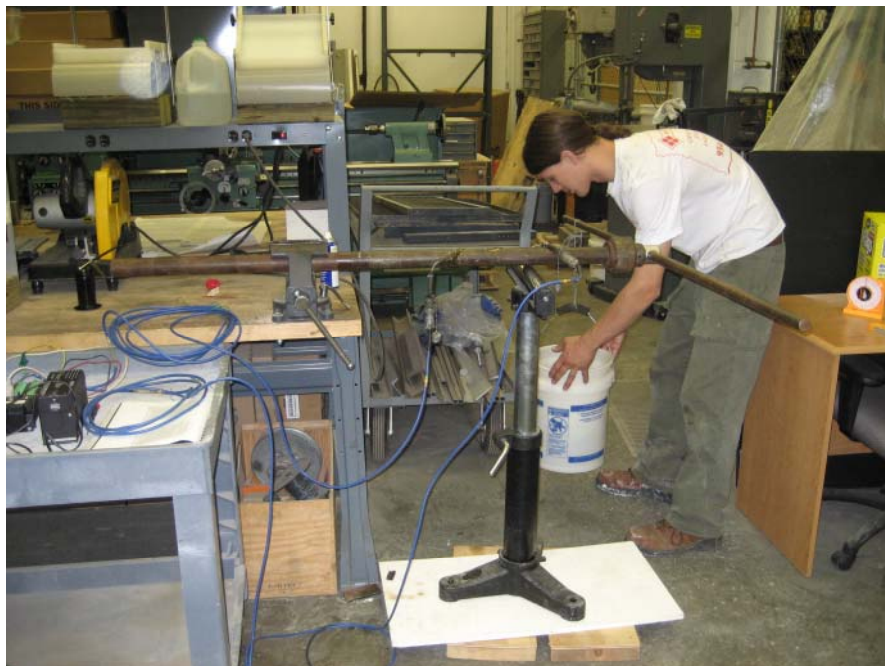
Figure 4.7 – Torque cell calibration equipment – Laboratory setup
