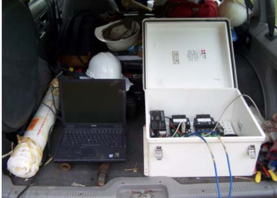
Figure 4.12 – Torque testing datalogger – Field set-up
