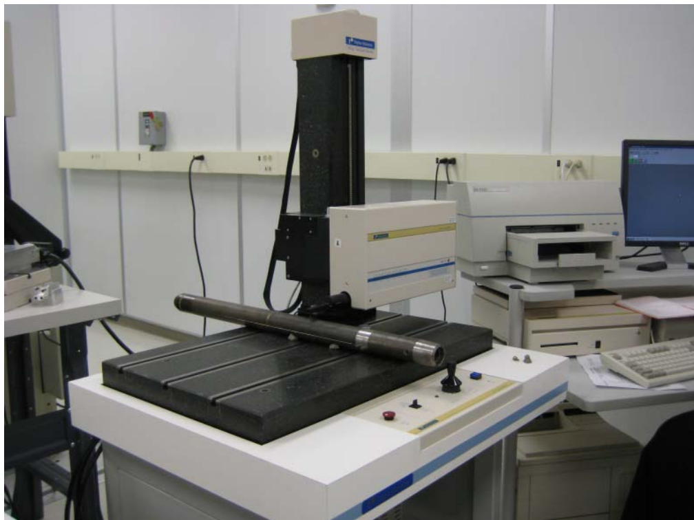
Figure 4.24 – SPT-T split-spoon sampler test set-up – Overall view
