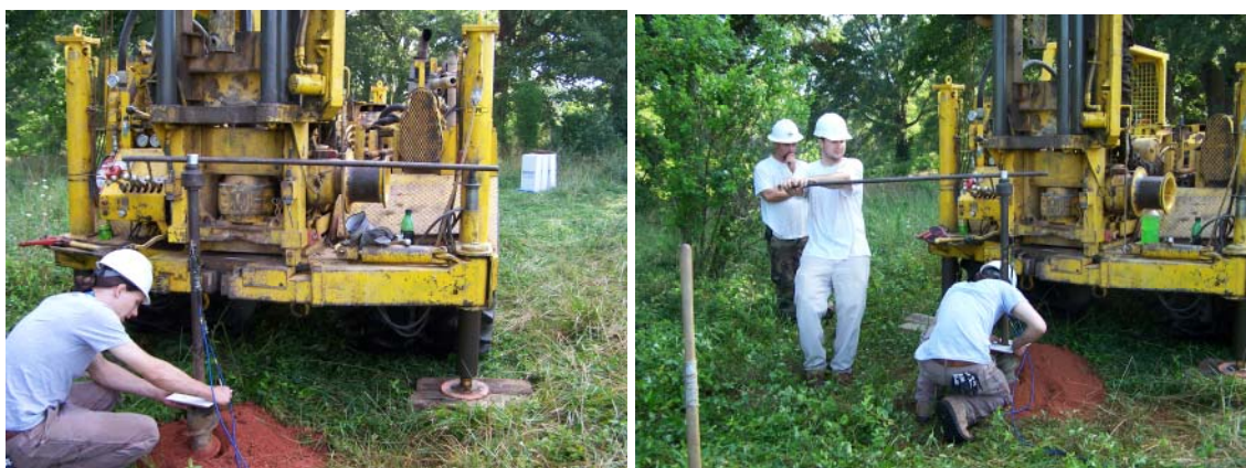
Figure 4.3 – Torque testing equipment – Insitu set-up
