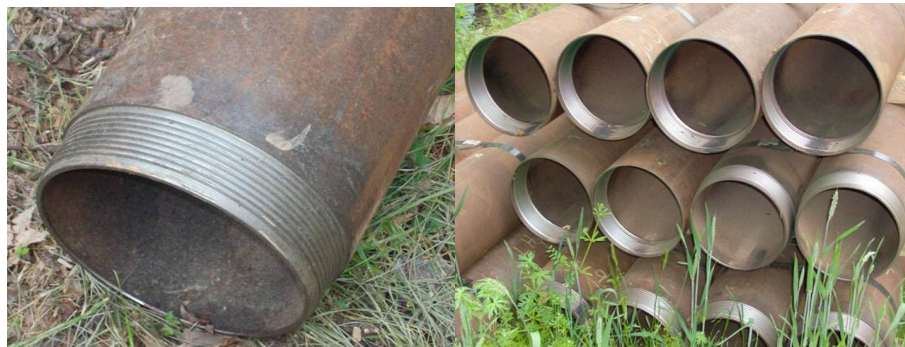
Figure 2.3: A Typical micropile threaded joint
