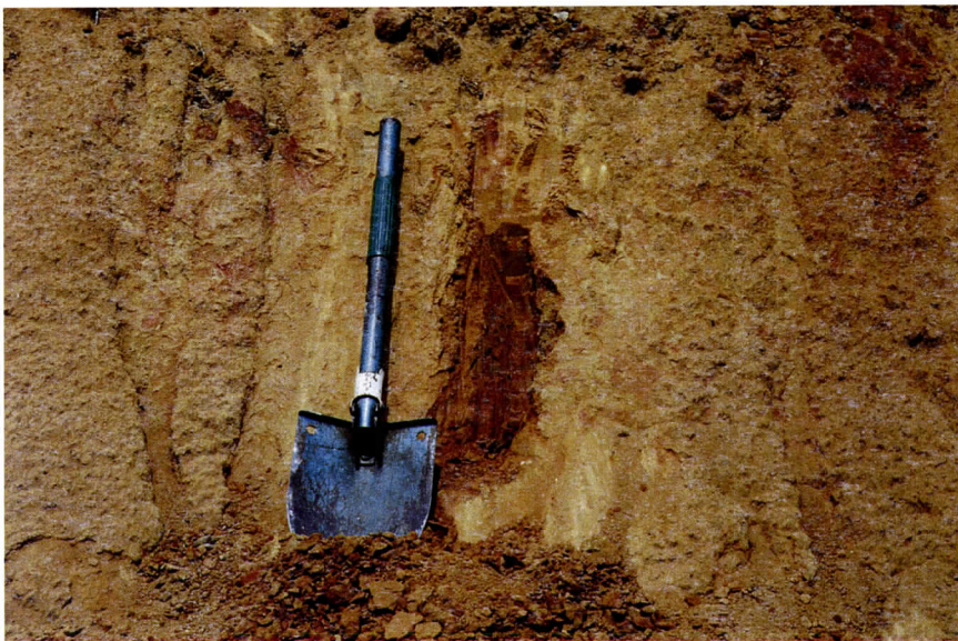
Figure 3. The Terrace deposits and upland sediments unit is typically reddish-brown. The 1-foot channel sample collected from this outcrop (located next to the shovel) contained 4.16 weight percent heavy mineral and 2.29 percent \text{TiO}_2 . The sample contained 0.05 weight percent +12-mesh material, 5.19 weight percent 12 x 30-mesh material, 60.85 weight percent 30 x 325-mesh material, and 33.91 weight percent -325-mesh material. This outcrop is located within the Bailey heavy-mineral deposits at an elevation of 88 meters (290 feet) above mean sea level.
