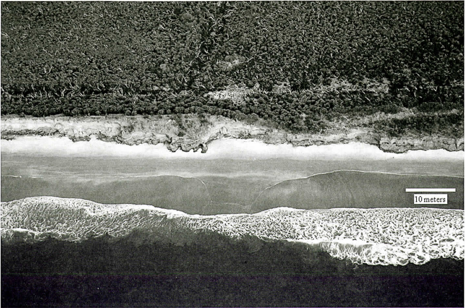
Figure 6. The bluffs and exposed marsh sediments on Morris Island are evidence of rapid shoreline retreat.
