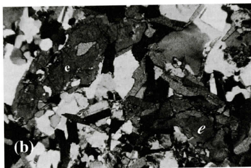
Figure 2. Photomicrographs of characteristic petrographic features of Persimmon Creek Gneiss. (a) Relict coarse, magmatic plagioclase [p] with modified grain boundary, surrounded by fine-grained, dynamically recrystallized quartz and feldspar. (b) Coarse, subhedral, zoned epidote [e].
