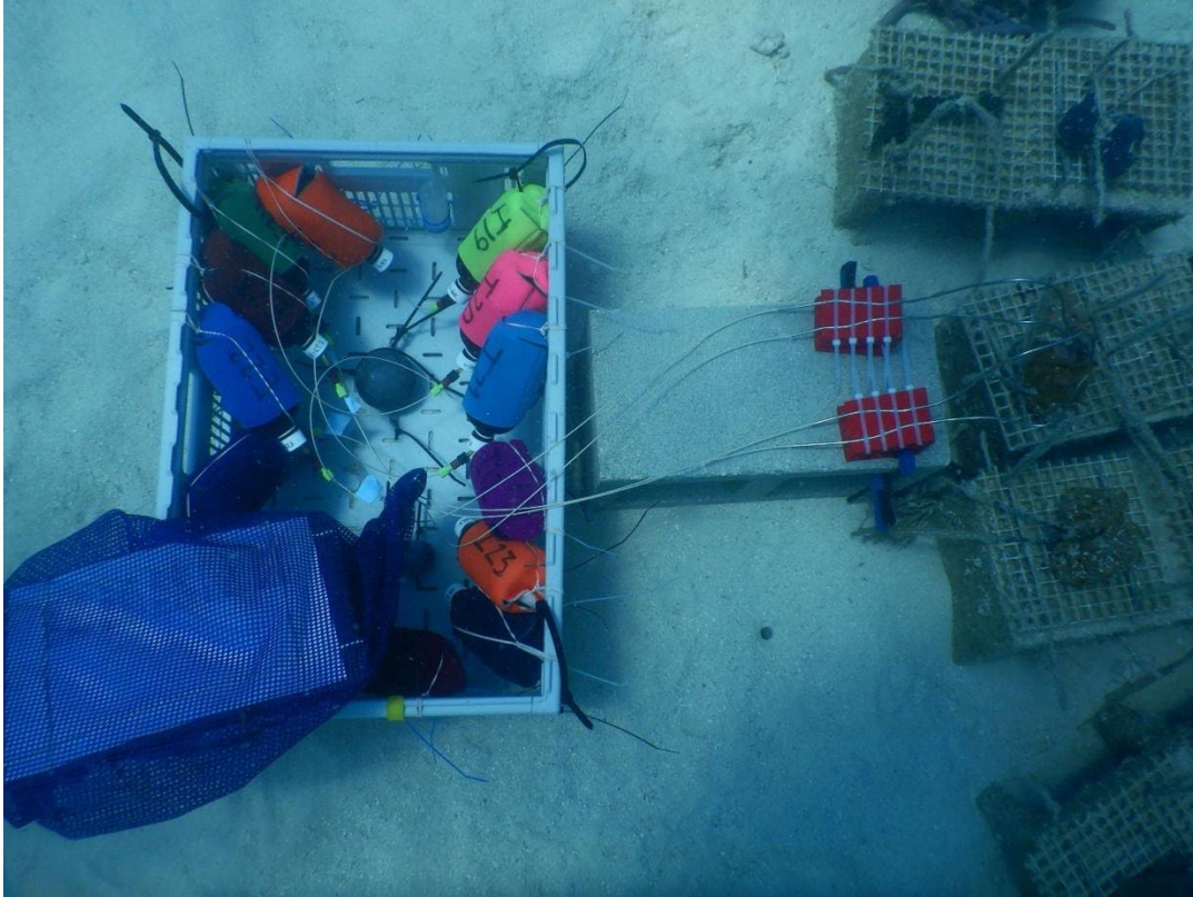
Figure 7 In-situ Vacusip setup and artificial reef. The basket contained a series of pressurized 250 mL bottles for sponge inhalant and exhalent seawater collection. The tubing was stabilized using the red blocks shown on the cinder block near the sponge to be sampled and positioned over the sponge osculum to collect exhalent water. Tubing for inhalant water was positioned in the basket to collect surrounding seawater. The tubing was plugged into the 250 mL bottles via syringe to initiate a vacuum to pull in seawater at a rate of \sim 1 \text{ mL min}^{-1} .
