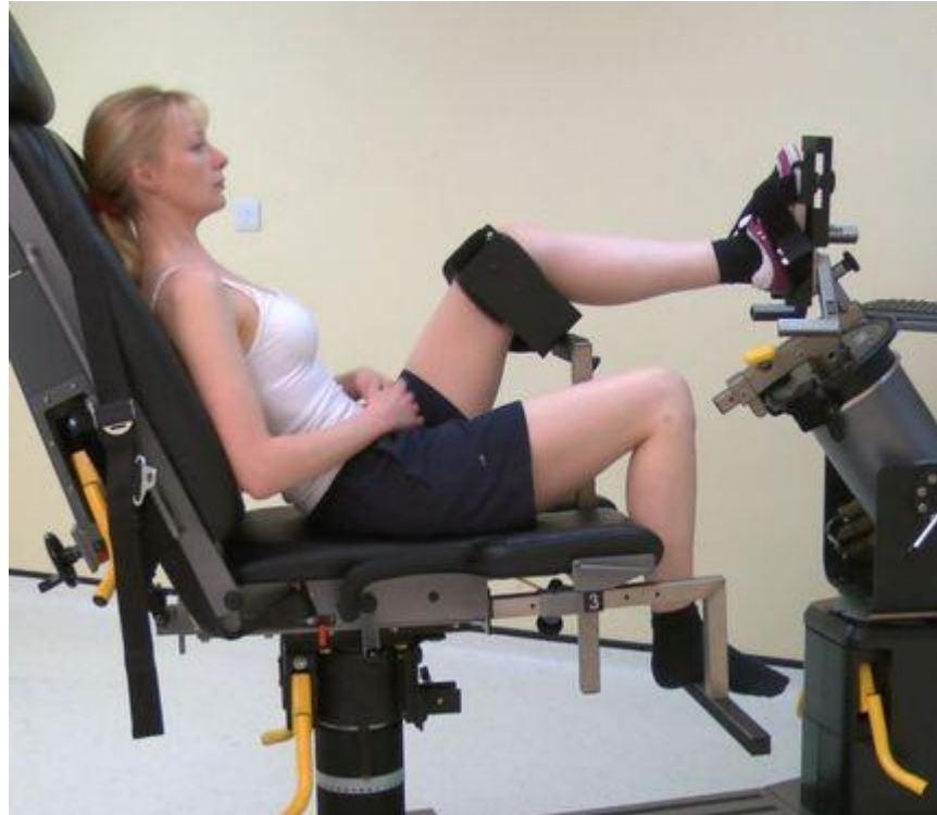
Figure 4. A picture of the body and dynamometer positioning during the strength portion of the testing sessions.
